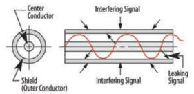
The table below illustrates the relative shielding properties of various shielding types. Notice as the shielding density increases there is a correlated increase in the shielding effectiveness value. The best shielding effectiveness value can be found in a rigid coaxial cable due to the solid tube construction of the outer jacket. In this type of cable the limiting factor for shielding effectiveness is the quality of the connector attachment.
