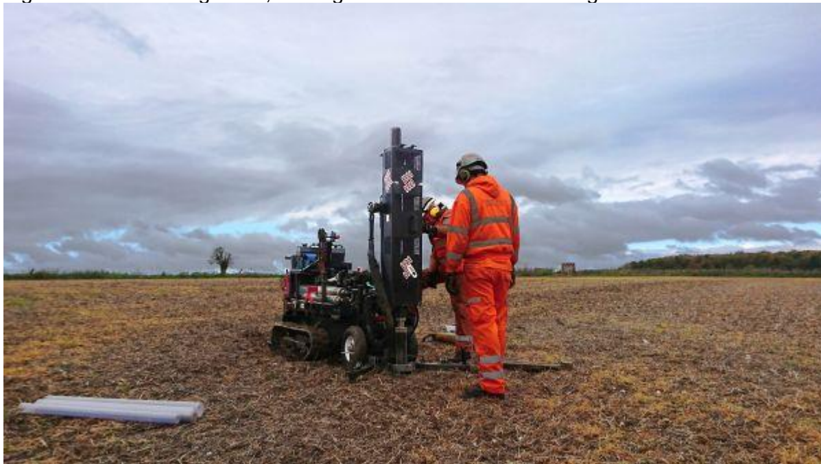
Figure 12: Dando Terrier rig in action at 5A looking north-west to anomalies 6A–7A, Strangways and Larkhill
