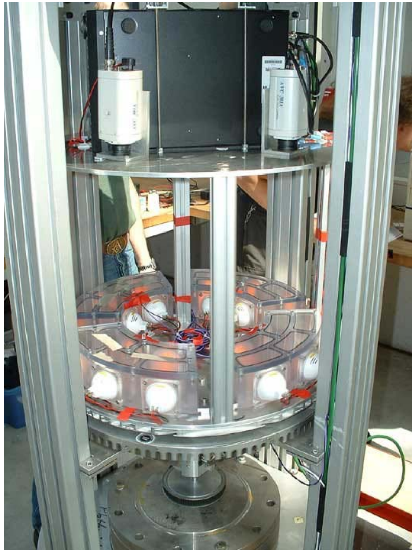
Fig. 21 Image depicts the turntable loaded with several fish tanks with individual illumination and camera observation
