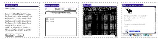
Ran some comms tests from the PDA: ping, portscan and an SSH connection. It's now getting seriously easy to manage a system via a suitably-connected hand-held device. I also ran another range test following the height increase, and I'm pleased to say that with an unobstructed path from the antenna the Billy can be found in our reception area, which represents over 100ft (about 33 metres). This through a mixture of walls and glass.
