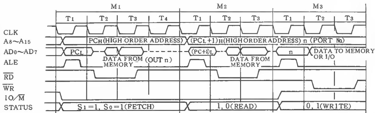
Fig. C-4 80C85 Basic System Timing
