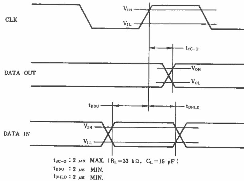
Fig. C-18  $\mu$ PD1990AC Command Input Timing Diagram
