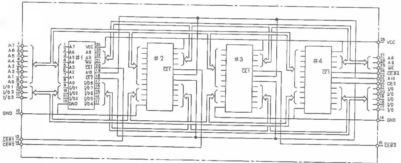
Fig. 4-2 Internal Wiring Diagram of RAM Pack
