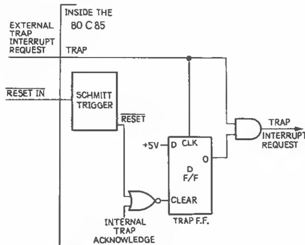
Fig. C-3 80C85 TRAP and RESET in Circuit
