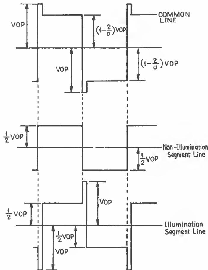
Fig. 4-36 LCD Waveform
