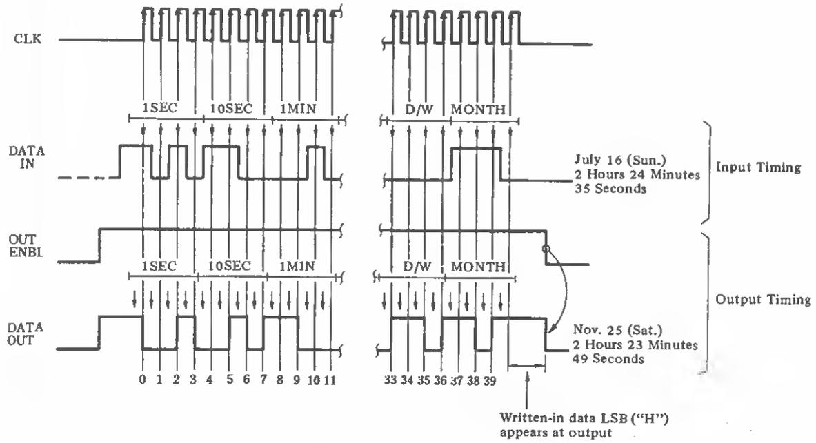
Fig. C-19  $\mu$ PD1990AC Data Input/Output Timing Diagram
