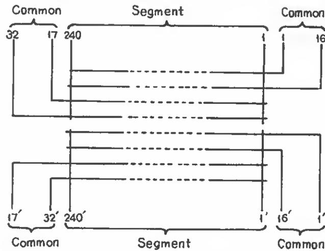
Fig. 4-32 LCD Electrodes
