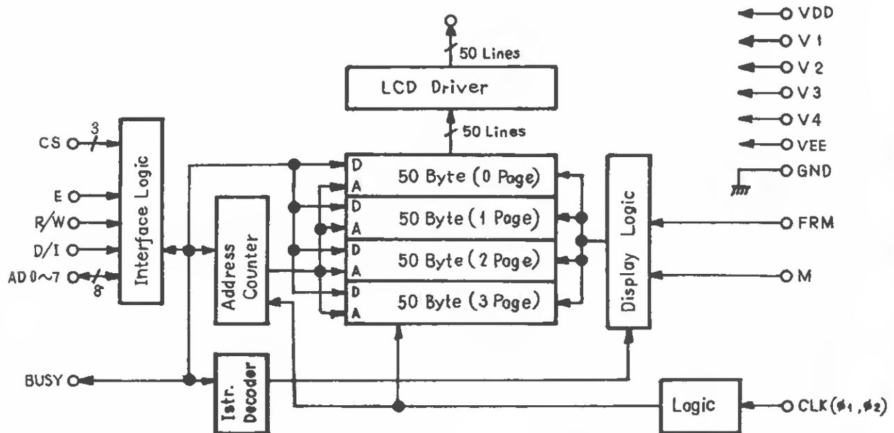
Fig. 4-35 HD44102 Internal Logic Diagram
