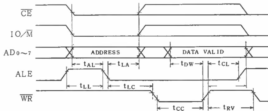
Fig. C-10 81C55 Read/Write Timing Diagrams
