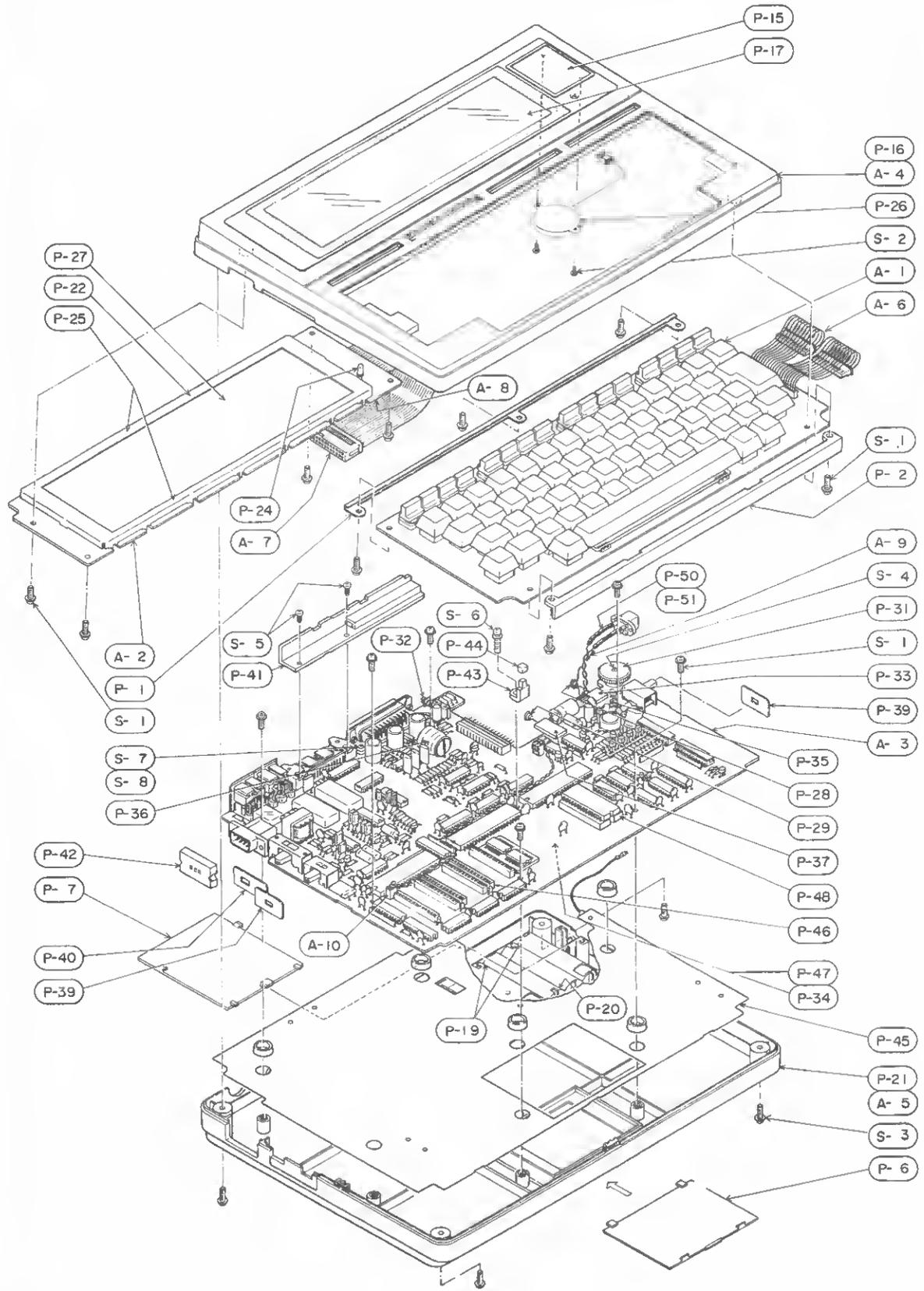
Fig. 6-1 Exploded View
