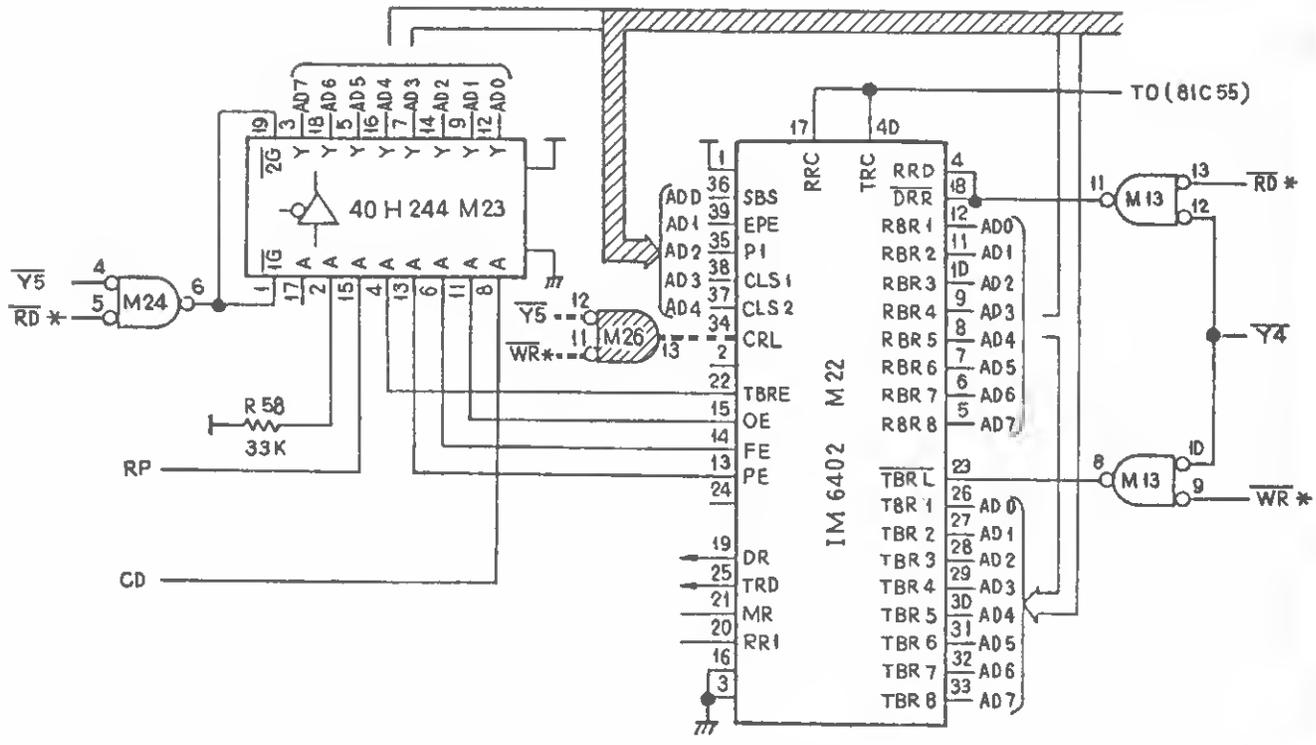
Fig. 4-20 Control Register Load Condition of IM6402
