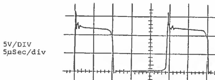
Fig. 4-38 Oscillation Waveform
