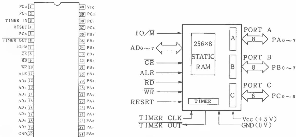
Fig. C-9 81C55 Pin Configuration and Block Diagram
