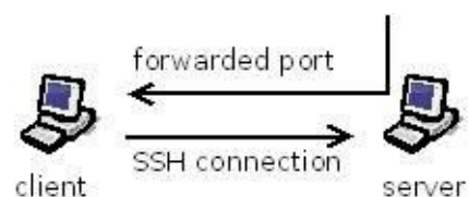
Figure 9-2: Remote Port Forwarding Data Flow
