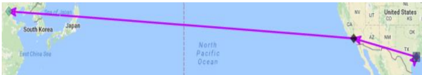
Figure 3b: US large bank to Italy but after hijack, traffic never arrives, seems to terminate in China.
