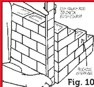
Do vertical joints first then horizontal ones using the full length of the trowel in a firm backwards action. The ruled joint is done by pressing about half the diameter of your home-made joint rule and drawing it the full length of the course. A recessed joint is made by undercutting the joints with a steel scraper with a protruding head the same size as the brick joints, or a block of timber with a nail protruding to the depth you want the joint to be.
