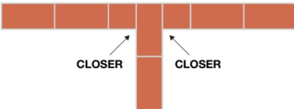
Broken Bonding occurs where the length of a brick wall is not equal to standard brick format sizes requiring for bricks to be cut to size and inserted. The cut bricks should not be less than a half brick.
