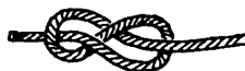
FIGURE EIGHT A stop knot which can be used to keep a line from coming out of a block.
