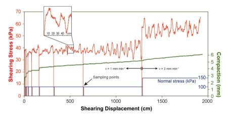
**Fig. 10.** Development of shear stresses and sediment compaction during the ring shear experiment 2 under normal stress of 100 kPa (0–1280 cm displacement) and 150 kPa (1280–1920 cm displacement). Note the shear stress heterogeneity evident during the entire experiment believed to have contributed to the variations in  $D_e$  distribution; v is the shearing velocity.
