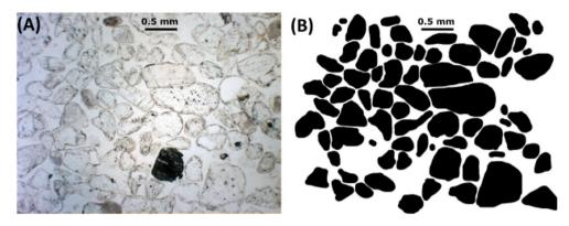
Fig. 9. An example of the sheared sediment collected at the end of experiment 1 after a shearing distance of 1280 cm. (A) Thin section of grains. (B) Black and white image analysis from thin section used to quantify grain orientation.
