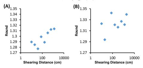
Fig. 6. Evolution of *round* (calculated on area of longest length; see Supplementary information for further details) in shearing-zone subsamples from (A) experiment 1 of Bateman et al. (2012) and (B) experiment 2.
