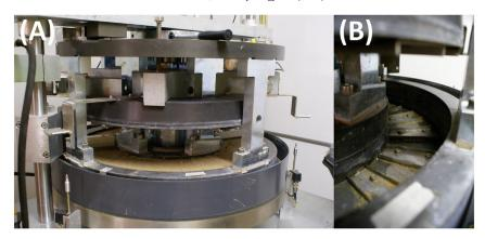
Fig. 1. The ring shear apparatus used for both experiments. (A) Apparatus loaded with sediment at end of the experiments. (B) The empty ring shear chamber showing the ribs on lid (top of picture) and in the base of the trough used to create shear stress.
