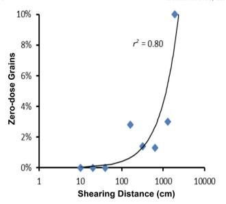
Fig. 4. Zero-dosed grains measured as a proportion of total number of grains accepted. Note final point underwent shearing at an extra  $50\,\mathrm{kPa}$ .
