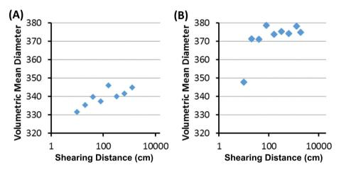
Fig. 7. Evolution of size in sheared subsamples from (A) experiment 1 and (B) experiment 2. Note the offset between experiments 1 and 2 attributed to inadvertent sorting during subsampling for artificial dosing.
