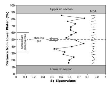
**Fig. 8.** Vertical distribution of  $S_1$  eigenvalues in the sediment at the end of experiment 1 after a shearing distance of 1280 cm. Note the relatively high eigenvalues in the shearing zone. Also shown is the distribution of main dip angles (MDA) of elongated grains at each depth, whereby a horizontal line is  $0^{\circ}$  dip and a vertical line is  $90^{\circ}$  dip.
