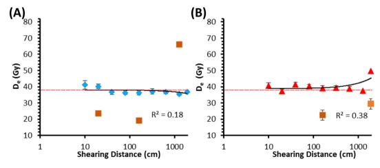
Fig. 3. FMM  $D_e$  component values (those representing > 10% of data only) from (A) unsheared and (B) sheared samples with distance sheared. Blue/red indicates dominant component and brown other components extracted. Dashed red line shows the initial gamma dose value. Note final point underwent shearing at an extra 50 kPa.
