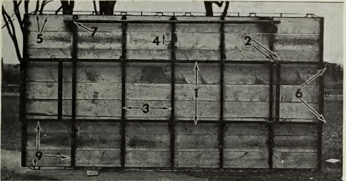
Figure 11—Bottom view of a combination rack showing steel stringers and cross joint.
