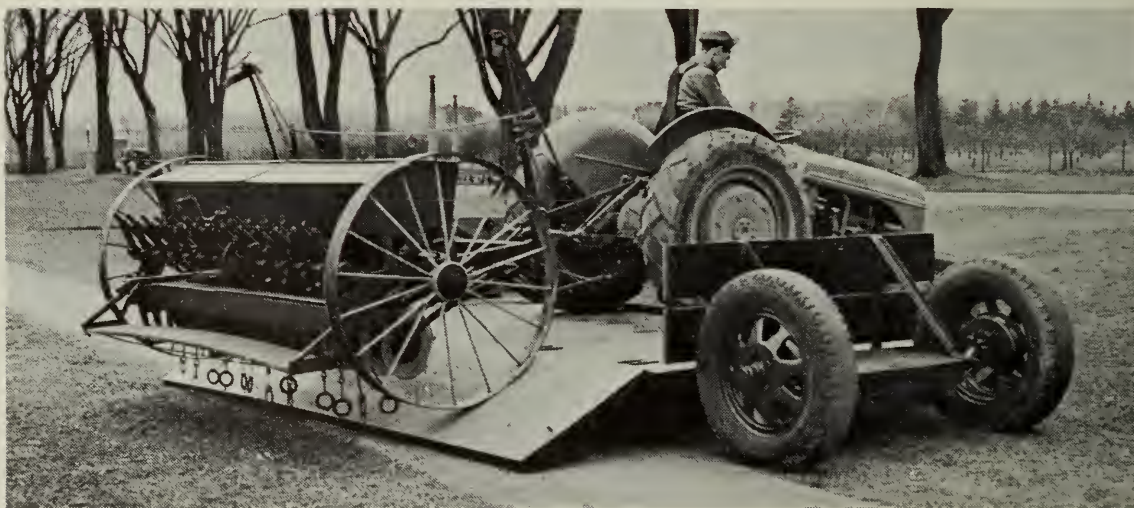
Figure 7—Light tractors can be driven across the transport wagon in loading equipment onto this low wagon.
