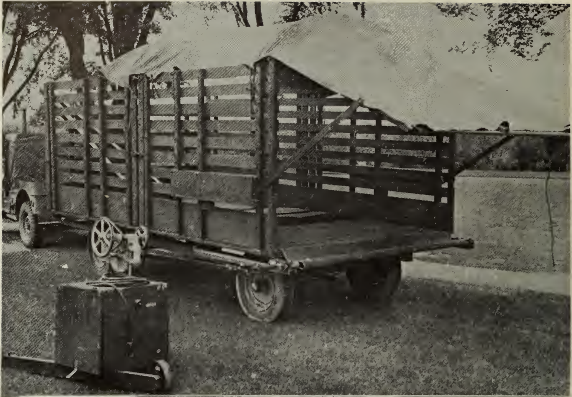
Figure 16—A canvas in the bottom of the rack can be used for unloading silage. A speed reduction unit is necessary to drive the canvas at the proper rate.
